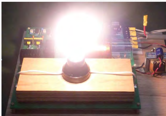
Takenaka Corporation used Q3D Extractor to determine the capacitance between electrodes in wireless power supply systems that are embedded in the walls and floors of buildings.
